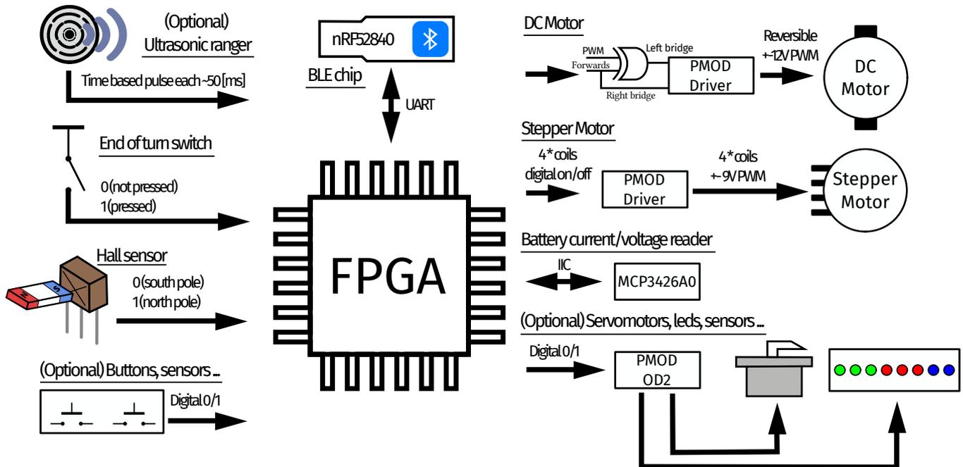
Figure 5 - Electronic Architecture
