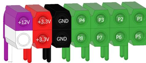
Figure 8 - PMOD pinning (header)
