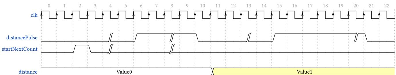
Figure 29 - Distance sensor timing diagram
