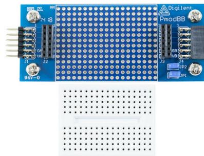
Figure 56 - PMOD Breadboard
