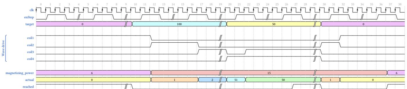
Figure 24 - DC Motor timings diagram
