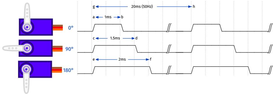
Figure 30 - Servo Motor Control pulse
