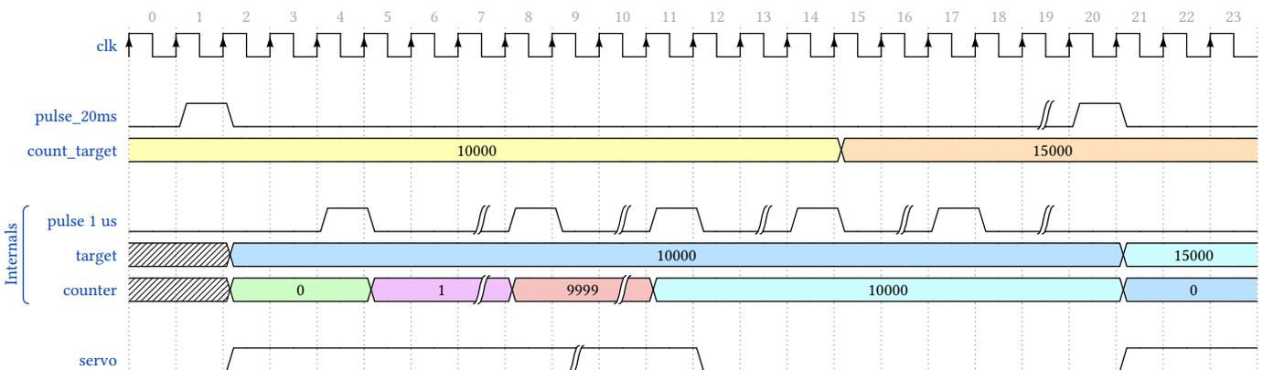
Figure 31 - Servomotors timing diagram
