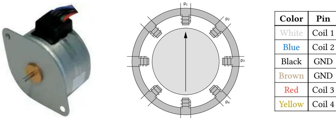
Figure 12 - Nanotec SP3575M0906-A Steppermotor, coils and pinning
