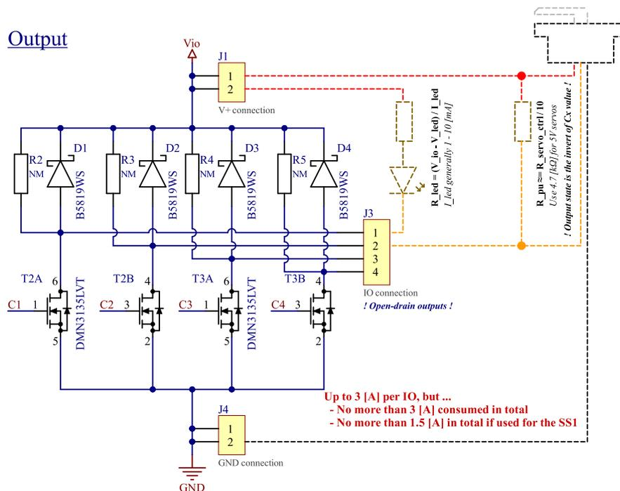
Figure 57 - Driving loads with PMOD-OD2
