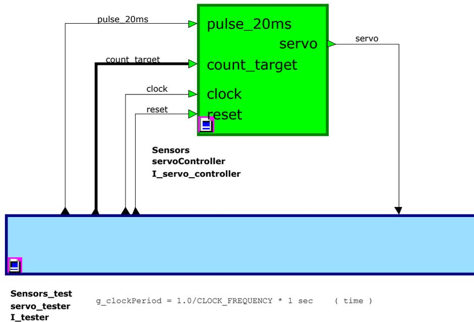
Figure 37 - Servomotor Testbench
