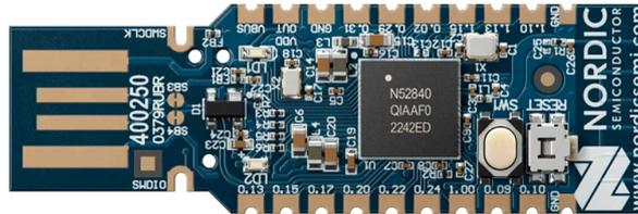
Figure 17 - NRF52840 Bluetooth Dongle
