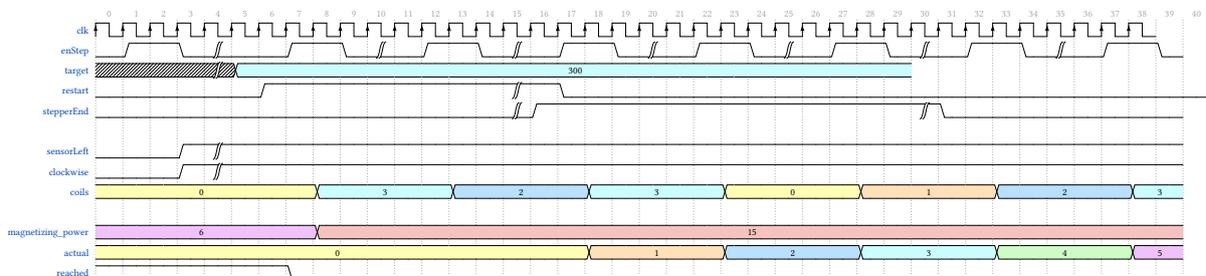
Figure 25 - Stepper restart sequence diagram
