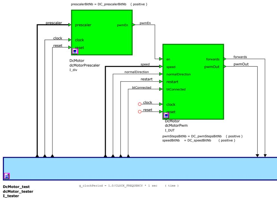
Figure 32 - DC Module Testbench
