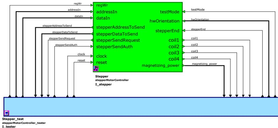
Figure 33 - Stepper Module Testbench
